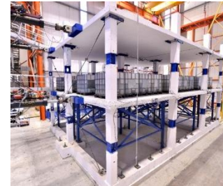
Flat-slab RC building
